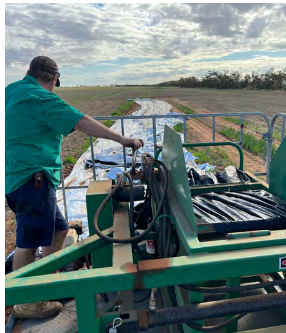
An example of a grain bag retriever used on-farm. Image: Marissa Shean.
